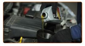
Replacement: engine oil and filter – SUZUKI BALENO Hatchback (EG). Tip from AUTODOC:
