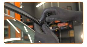
Remove the blade from the wiper arm.
