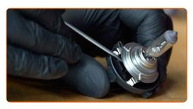
Replacement: headlight bulb – SUBARU IMPREZA Hatchback (GR, GH, G3).
