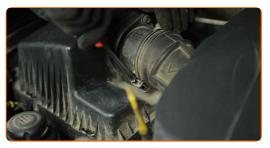
Disconnect the charger intake hose from the air filter housing.
