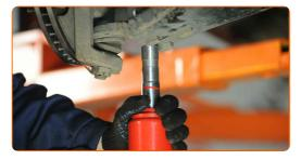
Tighten the lower fastening of the shock absorber. Use a combination spanner #19. Use a drive socket #22. Use a torque wrench. Tighten it to 125 Nm torque.
