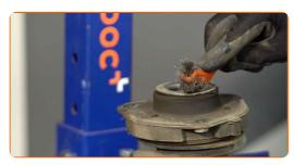
Remove the strut piston rod nut. Use a combination spanner #19. Use an adjustable wrench.
