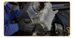
Connect the charger intake hose to the air filter housing.
