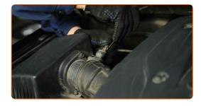
Loosen the fastening clamp connecting the air duct to the air filter housing. Use a Phillips screwdriver.
