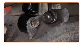
Attach the upper control arm to the steering knuckle. Use a crowbar.
