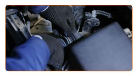
Unscrew the air filter housing fastener. Use a drive socket #12. Use a ratchet wrench.
