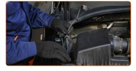
Remove the air filter housing.
