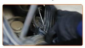
Detach the air intake hose clamp. Use a Phillips screwdriver.
