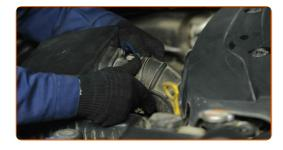
Fasten the clamp on the air intake hose. Use a Phillips screwdriver.
