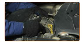
7 Release the air filter cover clips.
