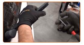
Press the clip. Use a flat screwdriver. Remove the blade from the wiper arm.
