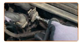
6 Unscrew the brake fluid reservoir cap.
