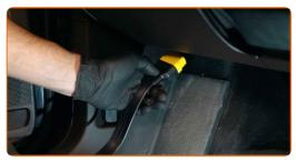
Put the parking brake system into service mode.
