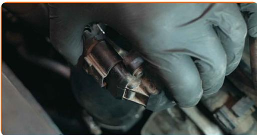
**63** Install the air duct.
