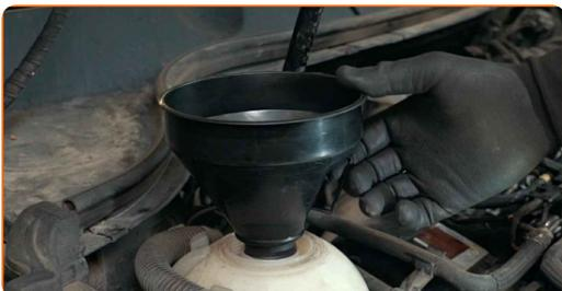
**66** Pour coolant in the coolant reservoir.
