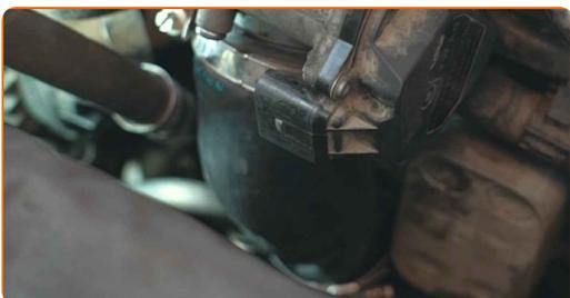
**60** Screw in the dipstick tube fastener. Use a combination spanner #10.
