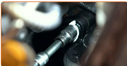
**43** Tighten the thermostat housing fasteners. Use a drive socket #10. Use a torque wrench. Tighten it to 9 nm torque.
