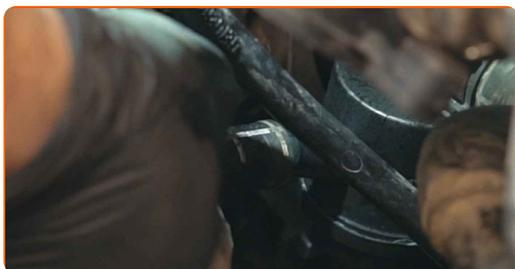
**48** Attach the clamp of the upper coolant hose. Use clic-R collar pliers.
