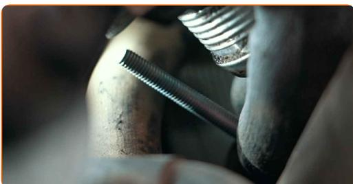
**13** Detach the throttle body from the intake manifold.
