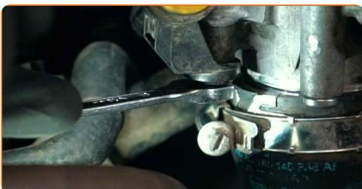
**61** Secure the fastener of the air intake duct. Use a drive socket #7. Use a ratchet wrench.
