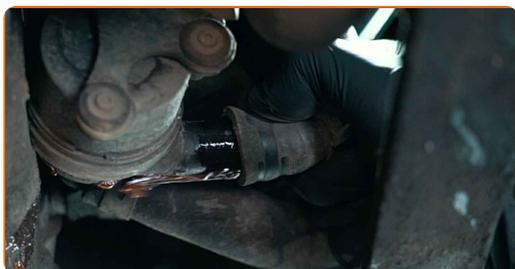
**20** Drain the coolant from the engine.
