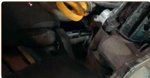
**7** Unscrew the dipstick tube fastener. Use a drive socket #10. Use a ratchet wrench.
