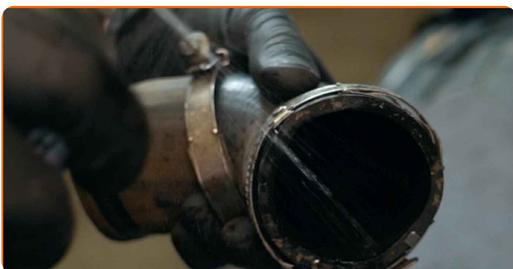
**59** Reinstall the air intake duct.
