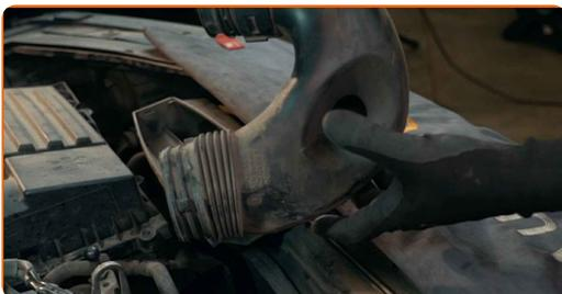
**4** Clean the throttle body fasteners. Use all-purpose cleaning spray.
