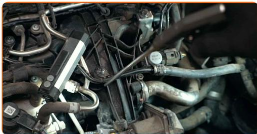
**5** Disconnect the throttle body connector.
