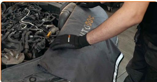
3 Remove the air duct.
