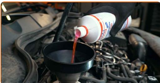
Replacement: engine thermostat – SKODA YETI (5L). Tip from AUTODOC:
