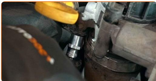
**8** Loosen the fastener of the air intake hose. Use a drive socket #7. Use a ratchet wrench.
