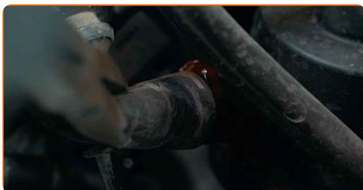
Replacement: engine thermostat – SKODA YETI (5L). Tip:
