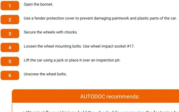
• Warning! To avoid injury, hold the wheel while unscrewing the fastening bolts. SKODA YETI (5L)
