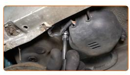
Remove the oxygen sensor housing cover.
