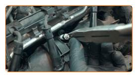
Tighten the glow plugs. Use the spark plug socket #10. Use a torque wrench. Tighten it to 18 nm torque.
