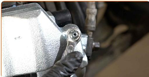
**25** Connect the brake bleeder kit to the brake bleeder screw.
