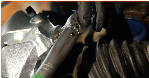
**23** Remove the brake hose clamp.
