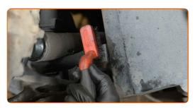
Install a new rod, tighten the fasteners. Use a combination spanner #18. Use a drive socket #18. Use HEX No.H5. Use a ratchet wrench.
