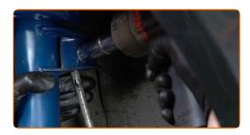
Unscrew the fasteners connecting the stabiliser link to the stabiliser bar. Use a combination spanner #18. Use XZN #6. Use a ratchet wrench.
