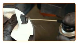
Clean the ABS sensor mounting seat. Use a wire brush. Use WD-40 spray.
