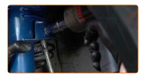
Unscrew the fasteners connecting the stabiliser link to the stabiliser bar. Use a combination spanner #18. Use XZN #6. Use a ratchet wrench.
