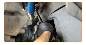
Tighten the fastener connecting the stabilizer link to the shock strut. Use a drive socket #18. Use a torque wrench. Tighten it to 60 Nm torque.
