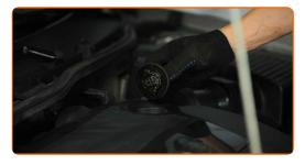
Tighten the oil filler cap.
