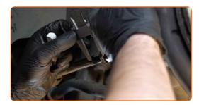
Loosen the lock nut securing the tie rod end to the tie rod. Use a combination spanner #23. Use a combination spanner #24.
