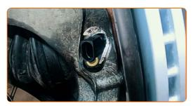
Tighten the fastener that connects the ABS sensor to the steering knuckle. Use HEX No.H5. Use a torque wrench. Tighten it to 7 Nm torque.
