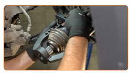
Install and tighten the drive shaft bolt. Use a drive socket #27. Use a ratchet wrench.
