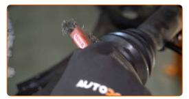
Detach the clamps of the CV joint boot. Use a crowbar.
