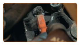
Unscrew the caliper bracket fastening. Use XZN #14. Use a tap wrench.
