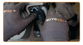
Treat the brake caliper piston. Use a nylon cleaning brush. Use a brake cleaner.
