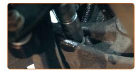
Remove the caliper bracket.
