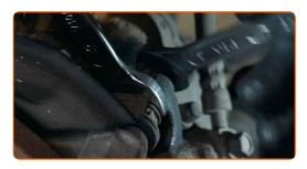
15 Remove the brake caliper.
