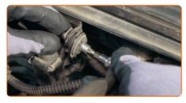
6 Unscrew the brake fluid reservoir cap.
