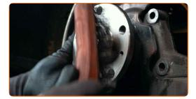
Treat the contacting surface. Use copper grease.
