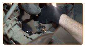
Unscrew the fastener connecting the brake pipe to the brake hose. Use a combination spanner #13.
