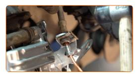
Screw in the fastener connecting the brake pipe to the brake hose. Use a combination spanner #13.
