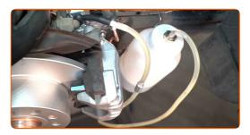
Undo the brake bleeder screw. Use a combination spanner #11.
