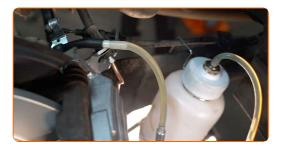
Tighten the brake bleeder screw. Use a combination spanner #11.
