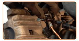
Remove the retaining clip of the parking brake cable. Use a crowbar.
