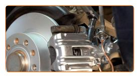
Clean the brake caliper fasteners. Use a brake cleaner.
