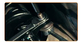
Tighten the fastener connecting the stabilizer link to the shock strut. Use a drive socket #19. Use a torque wrench. Tighten it to 65 Nm torque.
