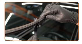
Remove the blade from the wiper arm.
