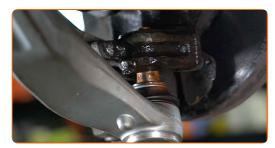
Screw the fastener connecting the ball joint to the steering knuckle. Use a combination spanner #18.
