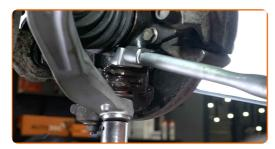
Remove the support from under the arm.
