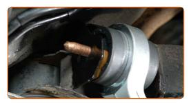
Screw the fastener connecting the control arm to the subframe. Use a combination spanner #18.
