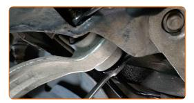
Unscrew the ball joint fastening to the steering knuckle. Use a combination spanner #18.
