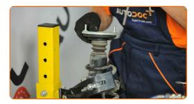
Tighten the shock strut piston rod nut. Use HEX No.H5. Use a drive socket #19. Use a torque wrench. Tighten it to 50 nm torque.
