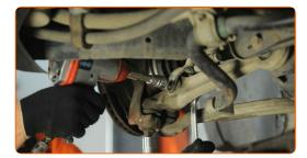
Remove the support from under the arm.
