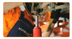
Tighten the fastening bolt that connects the shock absorber fork to the lower control arm. Use a combination spanner #18. Use a drive socket #18. Use a torque wrench. Tighten it to 90 Nm torque.
