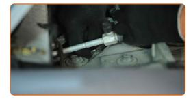
Unscrew the top fastening of the shock strut. Use a drive socket #13. Use a ratchet wrench.
