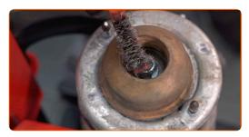
Remove the strut piston rod nut. Use a drive socket #19. Use a ratchet wrench.
