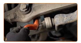
Unscrew the fastening bolt that connects the shock absorber fork with the lower control arm. Use a combination spanner #18. Use a drive socket #18. Use a ratchet wrench.
