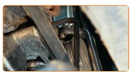
Place the serpentine belt on the crankshaft pulley.
