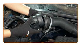
Tighten the MAF sensor fasteners. Use a drive socket #10. Use a torque wrench. Tighten it to 4 Nm torque.
