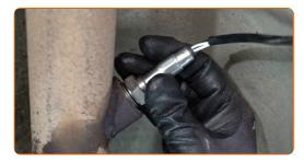
Tighten the oxygen sensor fastener. Use a 22-mm oxygen sensor socket. Use a torque wrench. Tighten it to 46 Nm torque.
