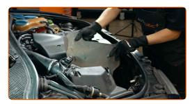
Screw in the fasteners of the heat shield of the air filter housing. Use a Phillips screwdriver.
