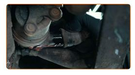
Drain the coolant from the engine.
