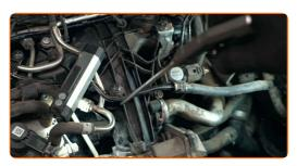
Disconnect the throttle body connector.
