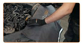
Remove the air duct.
