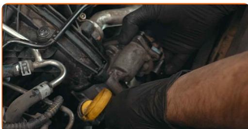
**56** Tighten the throttle body fasteners to the air intake manifold. Use Torx T27. Use a torque wrench. Tighten it to 14 nm torque.
