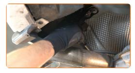
Make a mark on the crossmember and on the camber adjustment bolt.
