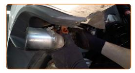
Clean the brake disk surface. Use a wire brush. Treat the surface where the brake disc contacts the wheel rim. Use copper grease.
