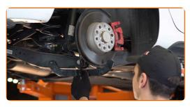
Remove the fastening bolt.
