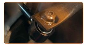
Remove the support from under the arm.
