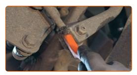
Unscrew the fastener connecting the stabilizer link to the stabilizer bar. Use a combination spanner #16. Use XZN #6. Use a ratchet wrench.
