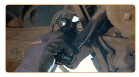
Tighten the stabiliser link fastener. Use a combination spanner #16. Use XZN #6. Use a ratchet wrench.
