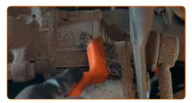
Unscrew the fastener connecting the stabilizer bar with the control arm. Use a drive socket #16. Use a ratchet wrench.
