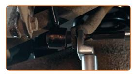
Tighten the fastener connecting the stabilizer bar with the control arm. Use a combination spanner #16. Use XZN #6. Use a drive socket #16. Use a torque wrench. Tighten it to 45 Nm torque.
