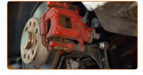
Unscrew the brake caliper fastening. Use a combination spanner #13. Use a combination spanner #19.
