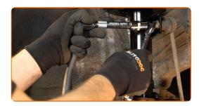
Unscrew the fasteners connecting the stabiliser link to the stabiliser bar. Use HEX No.H5. Use a combination spanner #16. Use a ratchet wrench.
