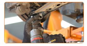
Disconnect the spherical joint from the arm.
