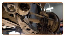
Clean the mounting seats and the thread of the suspension arm. Use a wire brush. Use WD-40 spray.
