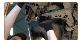
Remove the front fastener of the control arm. Use a drive socket #18.
