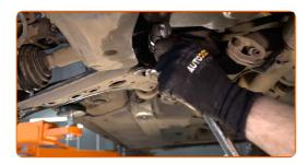
Unscrew the fastener connecting the ball joint to the suspension control arm. Use a drive socket #13. Use a tap wrench.
