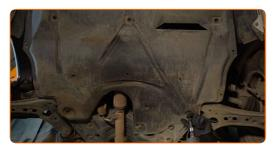
Remove the lower sound insulation.
