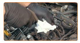
Remove the glow plugs. Use the spark plug socket #10. Use needle nose pliers.
