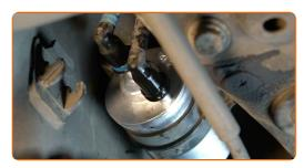
Take the fluid container away from under the fuel filter.
