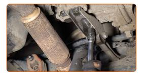
Unscrew the engine mount fastener that connects it to the subframe. Use a drive socket #16. Use a ratchet wrench.
