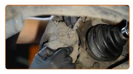
20 Install the brake caliper retaining spring.
