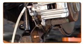
Secure the parking brake cable with the retaining clip.
