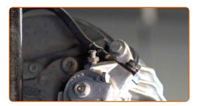
Undo the brake bleeder screw. Use a combination spanner #11.
