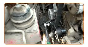
Remove the camshaft gear locking tool.
