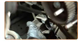
Unscrew the water pump fasteners. Use HEX No.H6. Use a ratchet wrench.
