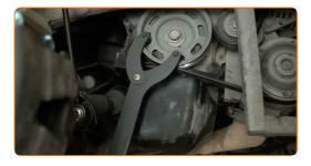
Tighten the crankshaft pulley fastener. Use 12-point socket No.21. Use a torque wrench. Tighten it to 90 Nm torque.+90°
