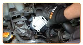
Tighten the ignition coil bolts. Use HEX No.H5. Use a torque wrench. Tighten it to 7 nm torque.
