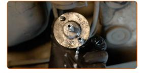
Disconnect the fuel supply lines from the fuel filter.
