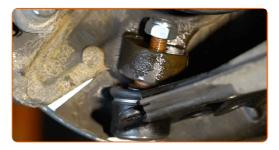
Screw the fasteners of the ball joint. Use a combination spanner #19.
