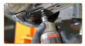
Disconnect the spherical joint from the arm.
