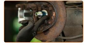
Install the new wheel hub with a bearing.
