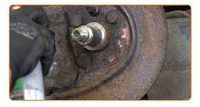
Apply special grease to the bearing assembly mounting seat.
