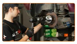
Screw the wheel hub lock nut.
