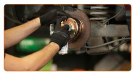
24 Install the brake disc.
