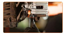
Remove the brake caliper.
