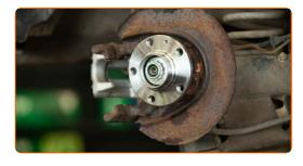
Tighten the hub. Important! Be sure to use new fasteners. Use drive 12-point socket #32. Use a torque wrench. Tighten it to 70 Nm torque.+45°
