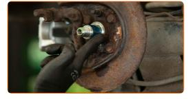
18 Install the new wheel hub with a bearing.
