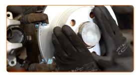
Tighten the brake disc fastening. Use Torx T30. Use a torque wrench. Tighten it to 4 Nm torque.
