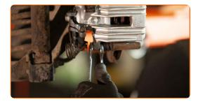
Remove the brake caliper.
