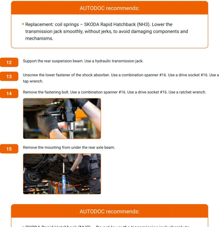
SKODA Rapid Hatchback (NH3) – Do not lower the transmission jack sharply to avoid damaging components and mechanisms of the car.
