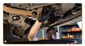
Replacement: engine oil and filter – SKODA Rapid Hatchback (NH3).
