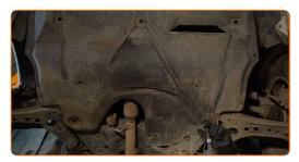
Remove the lower sound insulation.
