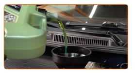
Replacement: engine oil and filter – SKODA Rapid Coupe (120G, 130G, 135G). Tip:
